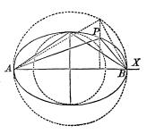
Hence, the angle formed by two supplementary chords of the ellipse will be within the angle formed by the corresponding supplementary chords of the circle, and will therefore be the greater angle. But the angle formed in the circle is a right angle; hence, the angle formed by the supplementary chords in the ellipse is obtuse.
